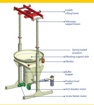
The Big Bag Unloader is engineered to discharge up to 2 ton supersacs, ensuring an automatic and complete discharge of the dry chemical without product compaction.
